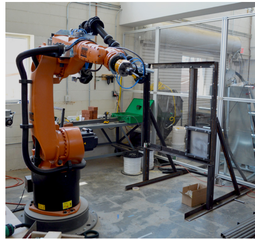
Figure 2: Metal forming stand used for both rigid and slip mounted forming.
